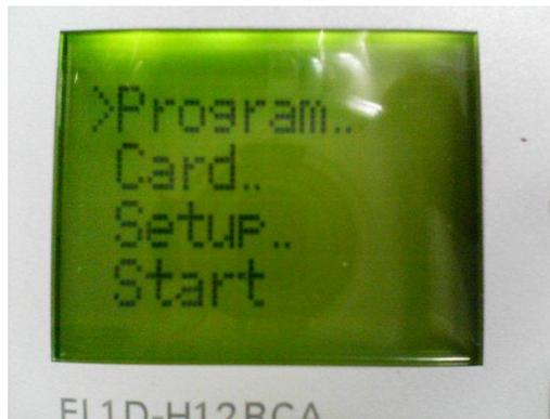
Use the down arrow key ▼ to point the cursor to ‘Start’, then press the ok button
