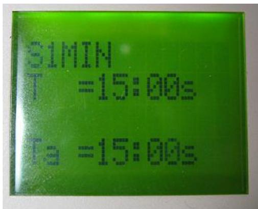
A timer will have the parameters ‘T’ and ‘Ta’. Using the up and down arrow keys ▲ ▼, the screen will cycle through all the blocks in memory.
